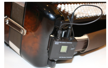
Figure 11 - Attach 5B Transmitter to bass strap.
