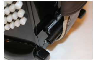
Figure 9 - Connector mounts under bass strap.
